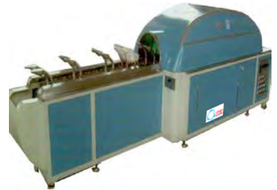
UHS-105 COMBINED UPPER CONDITIONING UNIT
