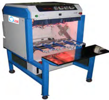
RINK-1 CEMENT DRYING UNIT
