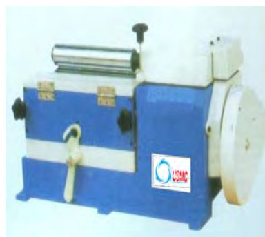
USZ-833 ADHSIVE (LATEX) CEMENTING M/C
